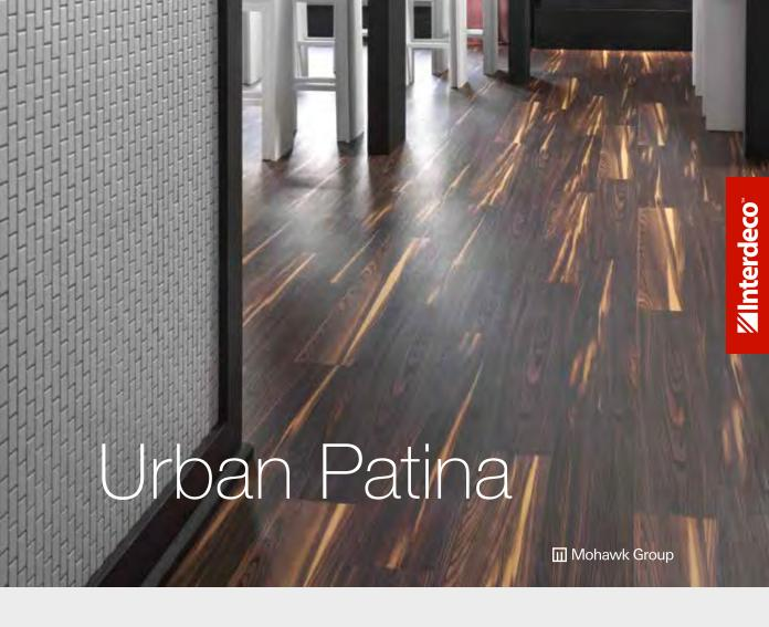
This highly versatile floor offers delightful innovation with never-before-seen visuals in fresh, unique colorways. The Uniclic® locking system is milled into all four sides, producing a tight connection that installs quickly. A commercial grade wear layer and M-Force™ Enhanced Urethane finish ensure performance under heavy commercial traffic. The adhesive-free construction works over existing flooring and saves time and costs.
