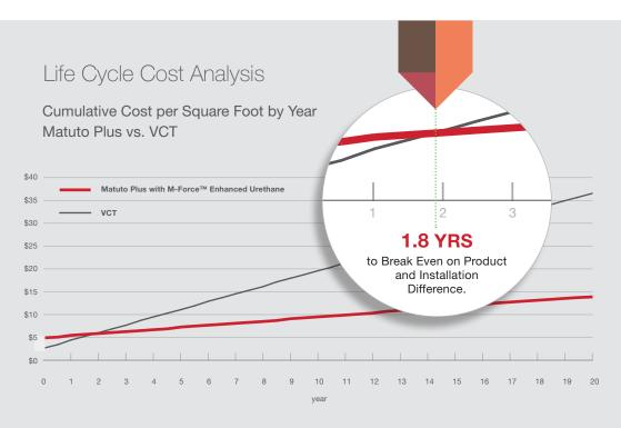
Matuto Plus enhanced resilient tile with M-Force™ Ultra Enhanced Urethane finish does not require polishing or waxing, which equates to significant cost savings over VCT. The payback occurs in as little as 2 years and compounds exponentially over the life of the installation.
